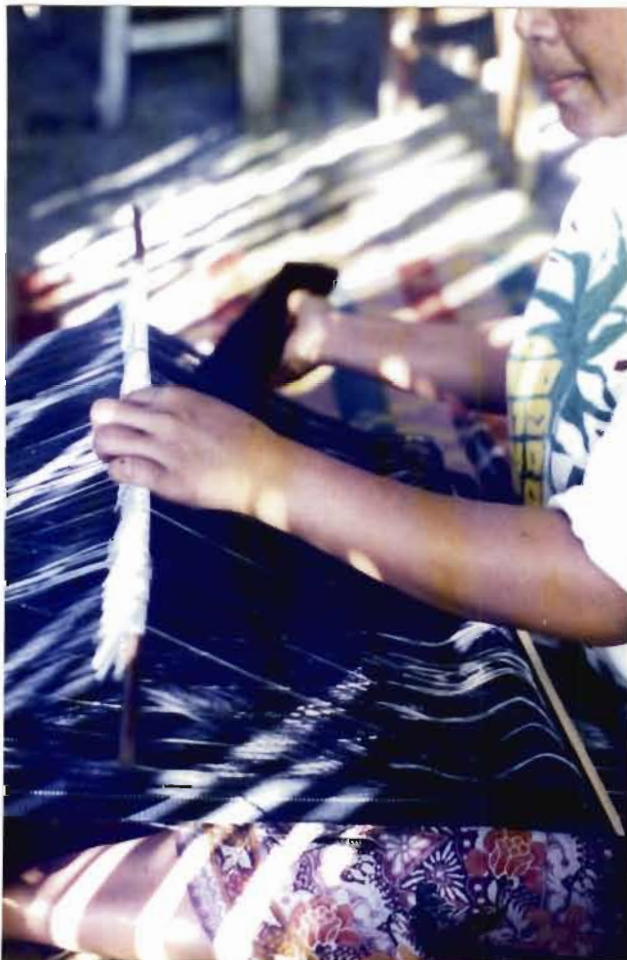
A Karen loom near Chiang Mai, Thailand. The sheds are determined by hand operated shafts.
