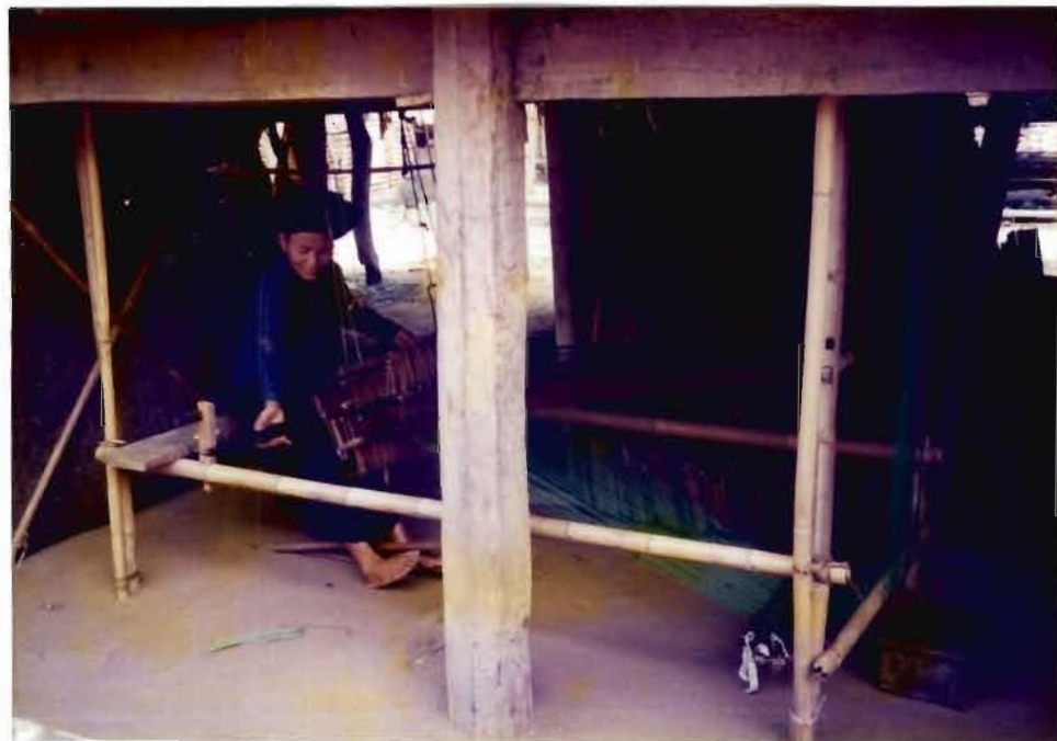
Tai Daeng frame loom in Ban Kang That, Houa Phan province, Laos. The warp is passed around the frame beams and knotted above the head of the weaver. This particular weaving has two warps for the weaving of a supplementary warp skirt called phasin muk . The ancestor of this design was probably woven on a backstrap loom. This loom is seen all over Laos and the northeast of Thailand.
