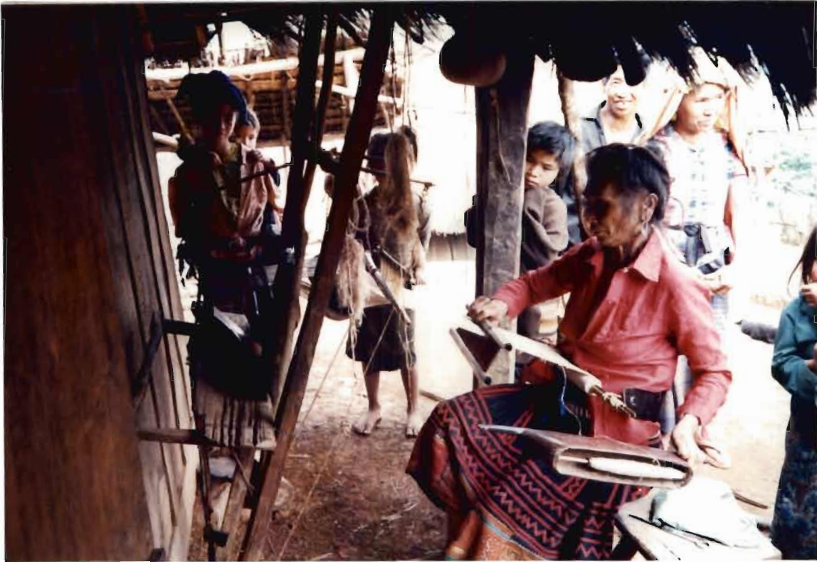
Hmong loom in Houa Phan province, Laos. The shuttle is very large with one edge shaped for beating in the weft. The comb is used as a warp divider.
