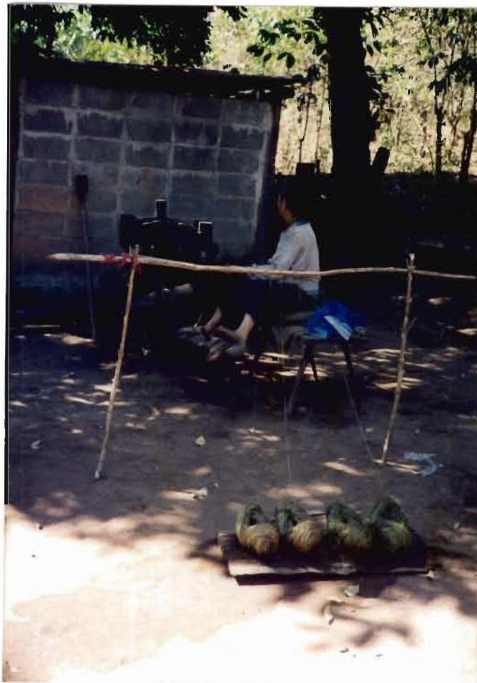
Twisting is done on a four spool, foot operated twisting apparatus. The wet bundles are laid on a log and passed over a frame to ensure smooth unravelling.
